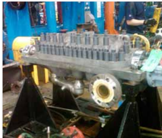
Control Rod Drive Pump at the test stand
